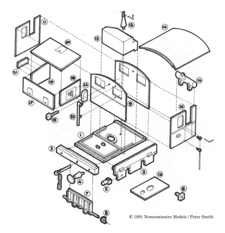
Before commencing construction, please read through the instructions and check through the parts. A dry run is perfectly feasible, but please follow the sequence of construction. Either low-melt solder, twin-pack epoxy resin or superglue can be used – if soldering, certain parts might still be better fitted with adhesive! If any parts are missing or damaged, contact us and we can arrange replacement. We can also help if you damage any parts during assembly.
